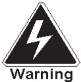
**THE COMPRESSOR ELECTRICAL CIRCUIT IS ALWAYS LIVE WHEN THE PLUG IS CONNECTED TO AN ELECTRICAL OUTLET**
